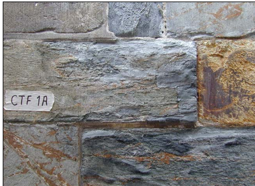
Example of documentation of test fields (field 1A at the north aisle of the choir). The upper picture shows a map of applied products, whereas the lower one shows the field after application (washes and mortars are visible on the picture)
