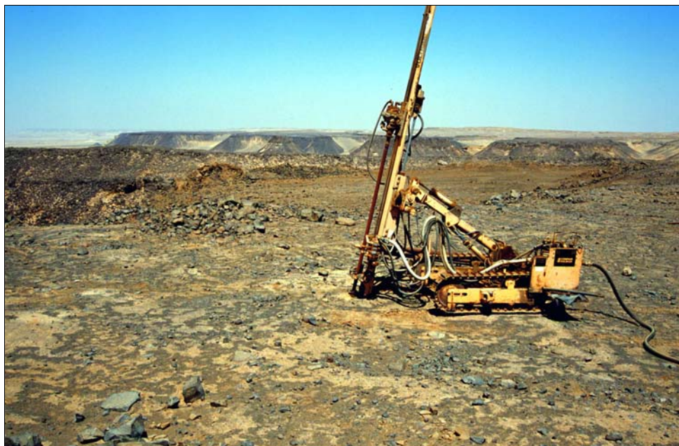
Fig. 20: Modern drilling just beside the ancient East quarry, either for testing basalt or for blasting (July 2003). Photo: James A. Harrell.
