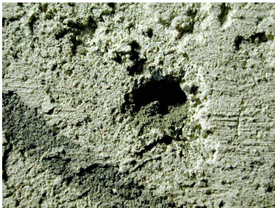
Another weathering form: Granular disintegration of aggregates (greenstone) in mortar. Width of field c. 10 mm
