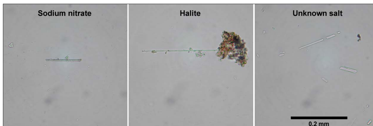
Microphotos of salts found on observation spot O.1. Left: Needle of sodium nitrate. Middle: Needle of halite. Right: Unknown salt (possibly aphthitalite). Pictures taken in normal light. The scale to the right applies to all three microphotos. Sample taken/analysed 2. June 2000
