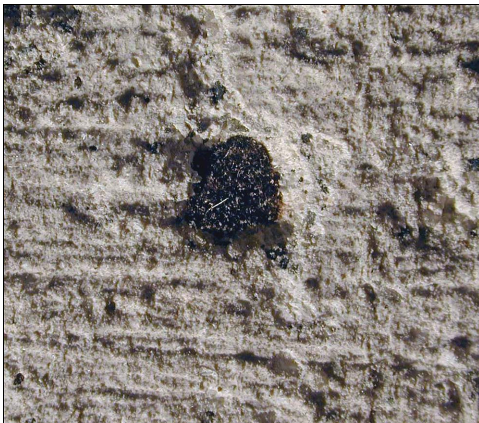
Observation spot O.1 on a dark aggregate grain. Note the tiny, white salt needle in the middle. Width of field c. 10 mm
