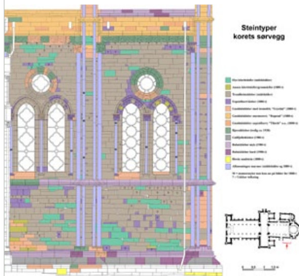
Figur 4. Nidarosdomen: Steintyper i korets sørvegg. Kart: P.Storemyr. Nidaros cathedral: Stone types at the south wall of the choir.
