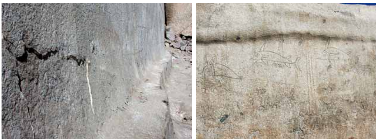
Figure 100: Salt weathering on the extensive quarry face shown on the picture above. Note that the dolphins and other drawings are becoming affected (photos: Per Storemyr 2006)
