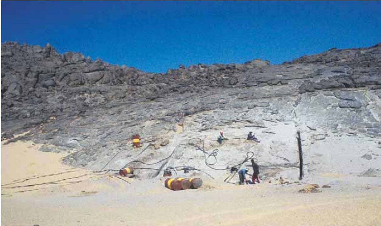
Figure 73: Modern trial quarrying in granite, Wadi Alaki (photo: Tom Heldal)
