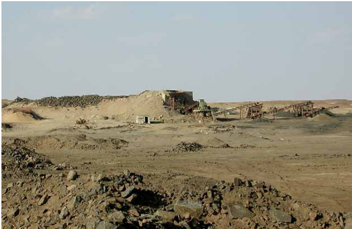
Figure 36: Basalt crushing machines by the modern basalt quarries at Widan el-Faras. The crushed basalt is used for e.g. road building (photo: P. Storemyr 2005)
