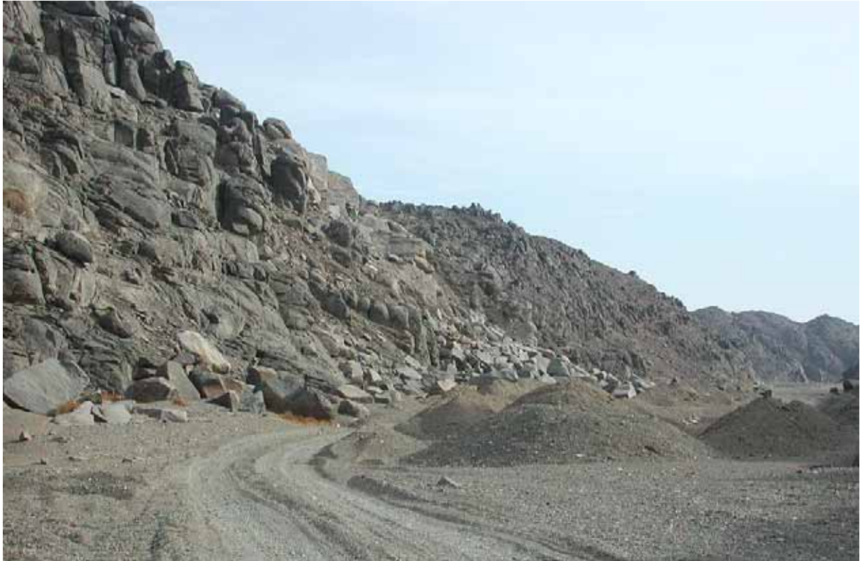
Figure 68: Current modern quarrying in the Eastern Desert is often taking place in an ad hoc manner, locating good blocks and targeting these instead of opening true quarries. This picture is taken in the south-central portion of the Eastern Desert, west of the Barramiya area. The stone extracted is granite (photo: Per Storemyr 2003).
