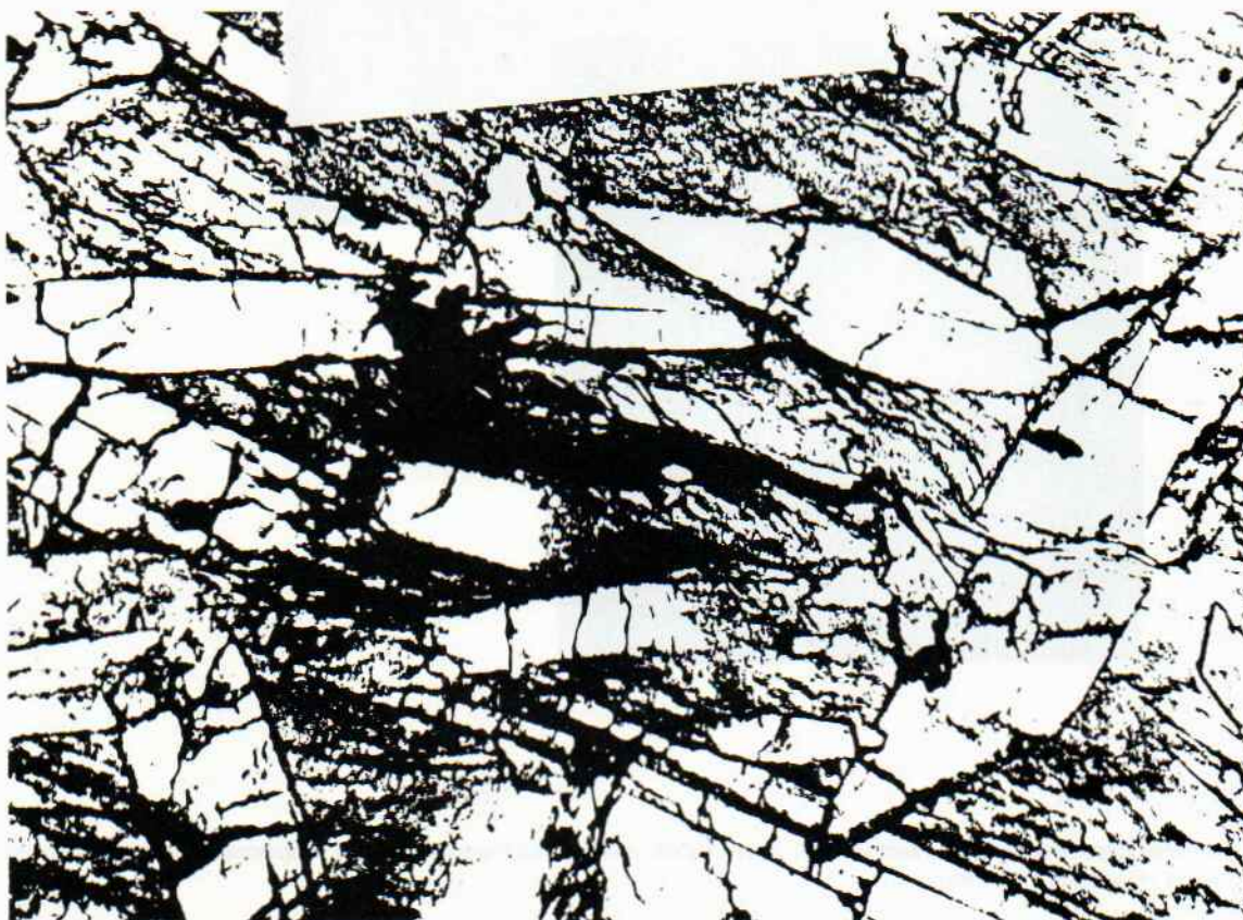
Fig. 7. Thin-section photograph from a deteriorated Grytdal soapstone sampled at the Nidaros Cathedral. Notice the cracks penetrating the amphibole grains.
